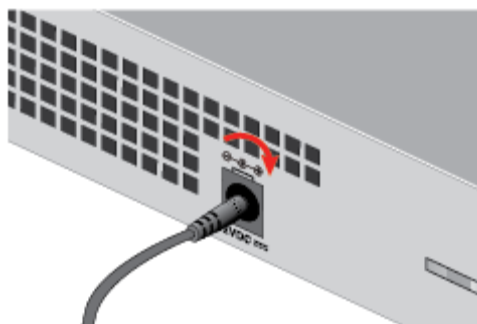
Figure 30. Locking the Power Cord for the DC Power Supply Socket
