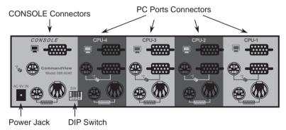
Note: Above panel description uses the 4-port model 098-8040 as an example different models will have different types and different numbers of connectors but the layout is similar. Please refer to the section "Specification" in page 4 for detail. And Rear Panel Description
