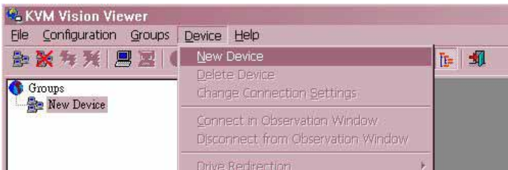
Figure 5-17. Create a new Device
