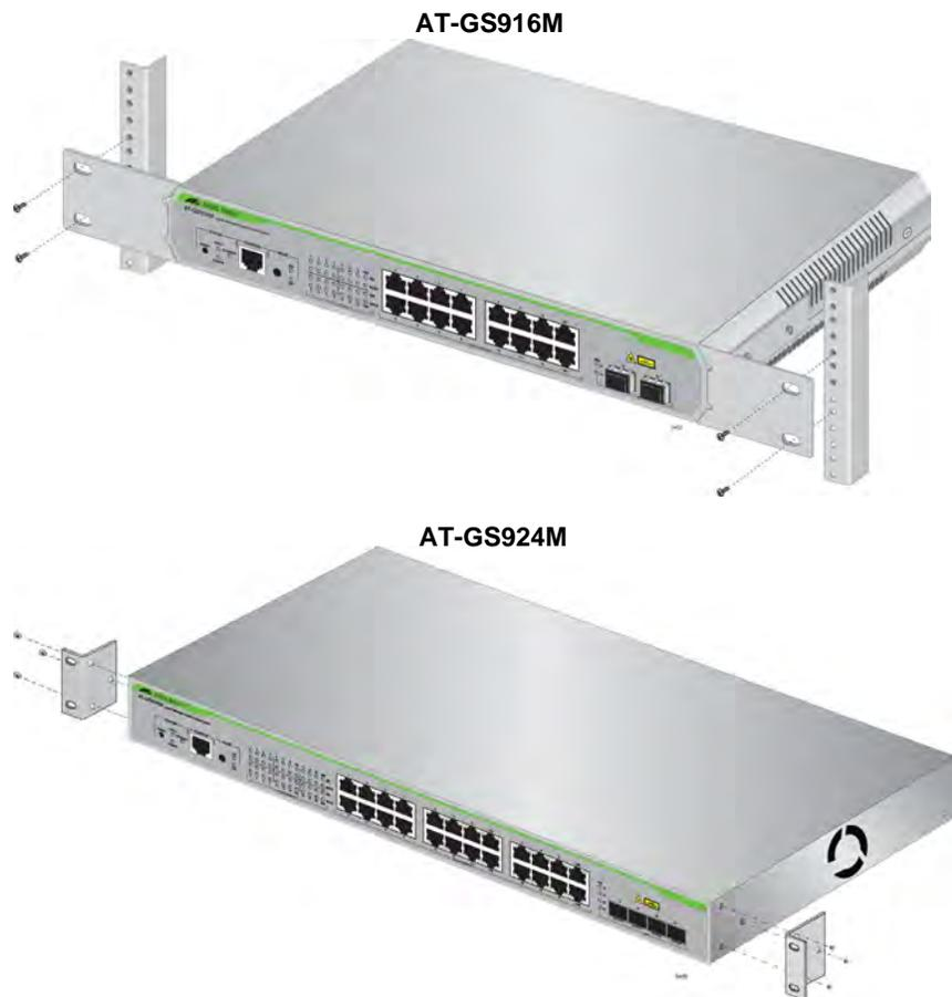
Figure 10. Attaching the Rack-Mount Brackets to the Switch
