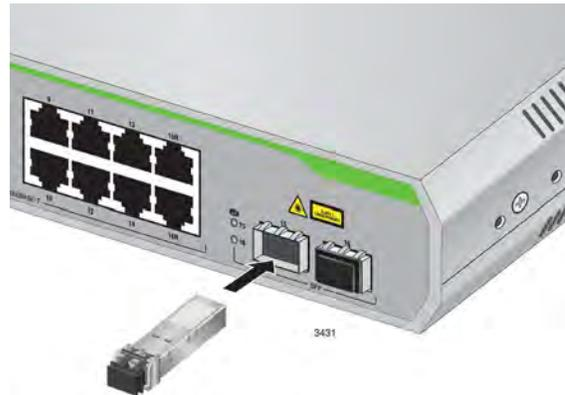
Figure 13. Inserting the SFP
