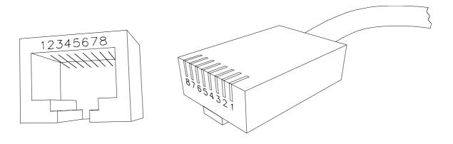
**RJ-45 Connector and Cable Pins**
