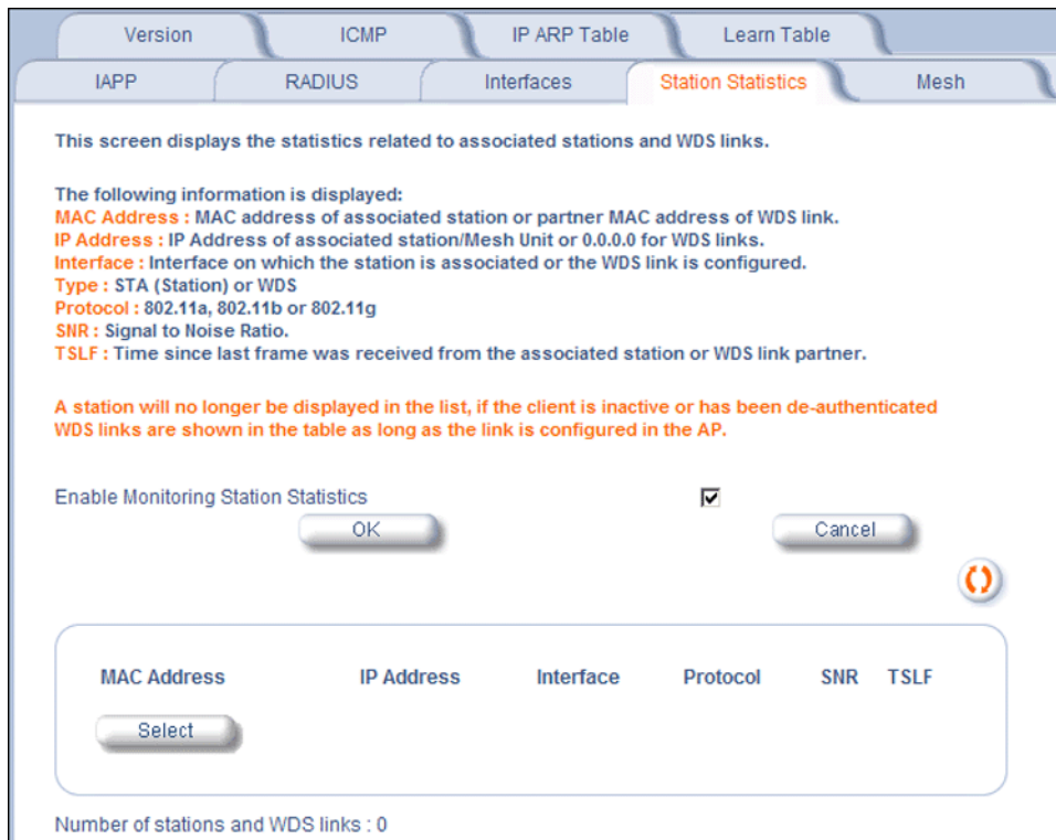
Figure 5-9 Station Statistics Monitoring Tab
