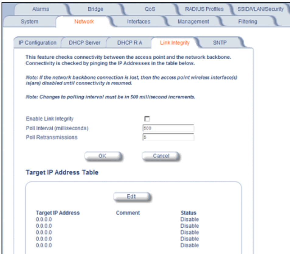
Figure 4-7 Link Integrity Configuration Screen
