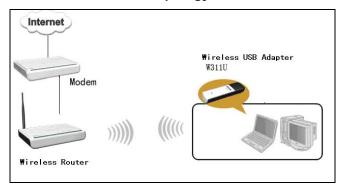
In this mode, W311U serves as a client to receive the wireless signals to access the Internet.
