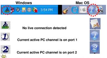
The KVM Switcher Software supports both the Windows and the Mac OS operating systems. For other OS platforms such as Linux, you can still use the keyboard hotkey - ScrLk + ScrLK - to switch PC.
