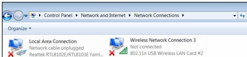
**Step2.** To configure the wireless network adapter's IP address, right click wireless network connection on the above screen and then refer to chapter 3.1-step 4 and 5 for further configurations.
