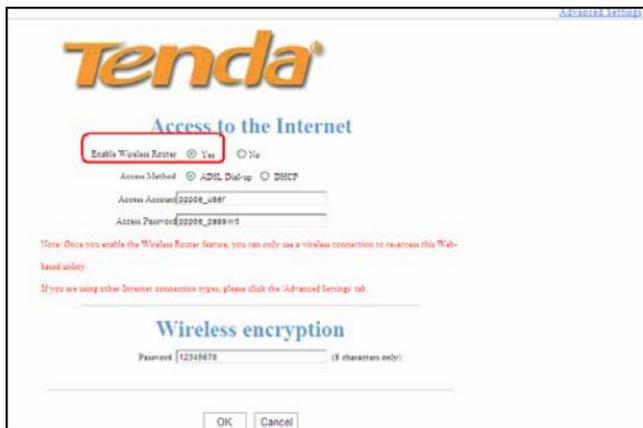
**NOTE:** *In Wireless Router mode, the LAN/WAN port functions as a WAN port only. So once enabling this mode, you can only use a wireless connection (a computer with an installed wireless network adapter) to re-log in to the device's Web-based utility. To wirelessly connect to the device, you need to set your computer to "Obtain an IP address automatically" (Refer to appendix 1) or configure a valid IP for your computer.*
