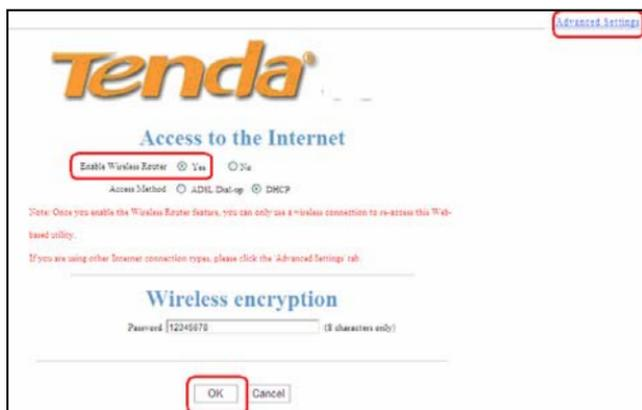
To do this, click on the “Yes” button next to where it says “Enable Wireless Router”, and then click on the “OK” button on the screen above to wait for device to restart.
