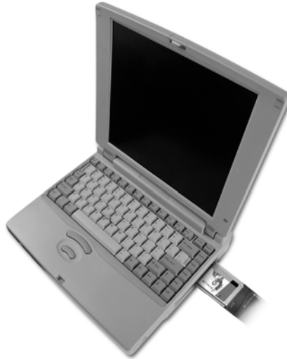
Figure 2-7 Insert the ORiNOCO Wireless Client into the Laptop
