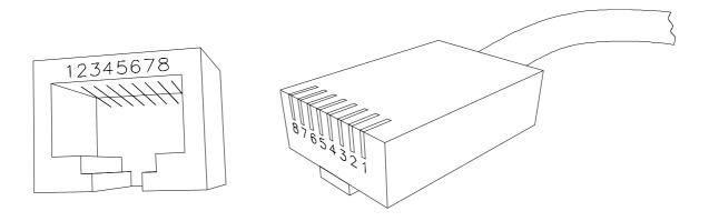
**RJ-45 Connector and Cable Pins**
