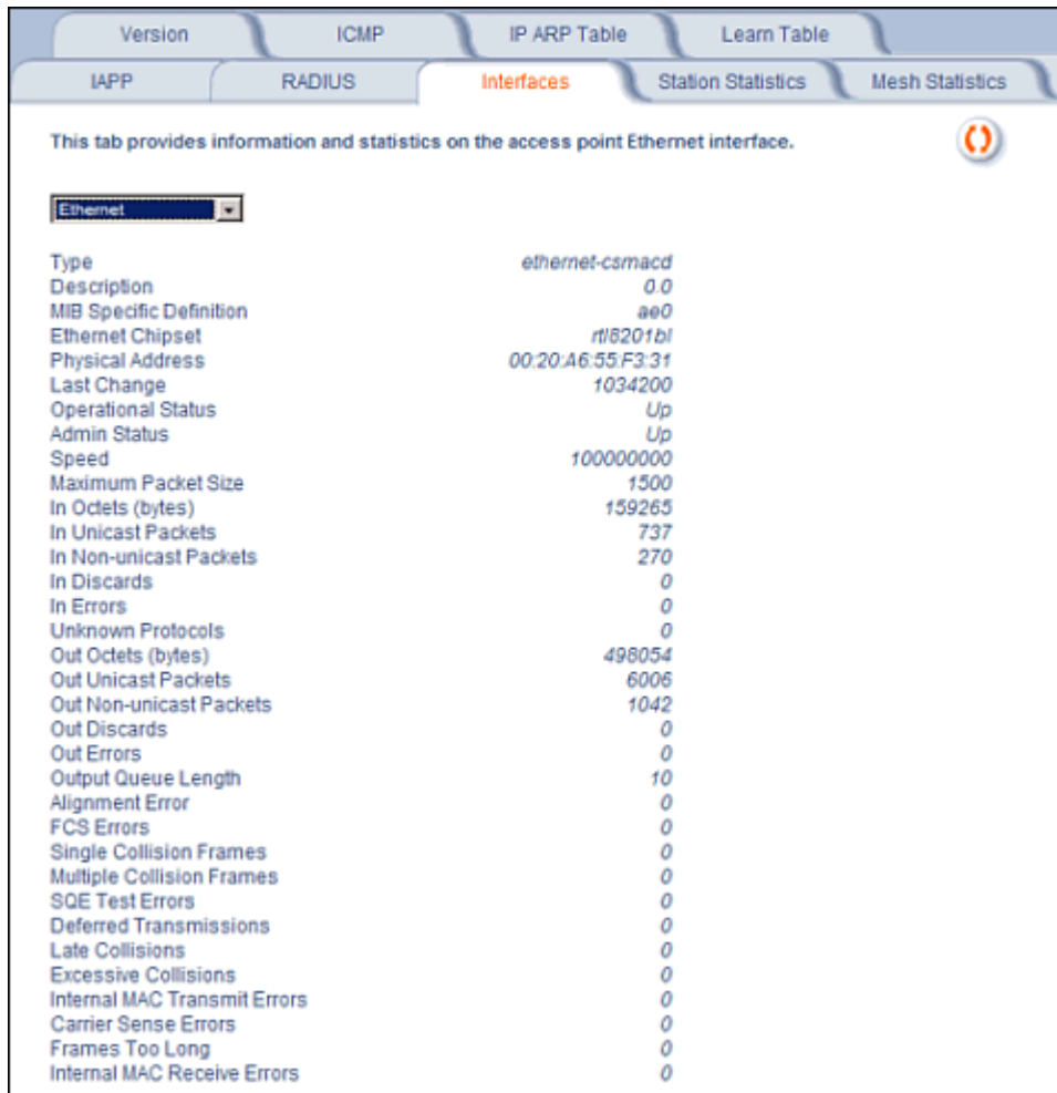
Figure 5-8 Interface Monitoring Tab (Ethernet)
