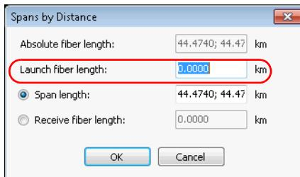
5. Select whether you want to enter the span length or the receive fiber length, then enter the appropriate value. The other value is updated automatically according to the value you have entered. If no event is present at the new position of the span end then, it automatically creates a new event.
