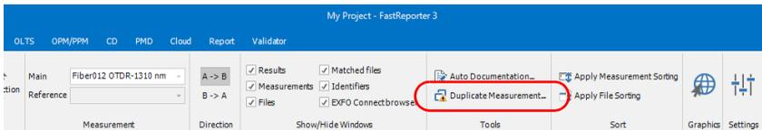
The files are analyzed and the result appears on-screen. The duplicate measurement tool will display the unit serial number, test date/time, identifiers, and filename details.
