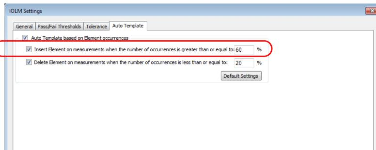
5. If you want to remove elements, select the corresponding option and enter the percentage value of occurrences under which the element must fall to be removed from the measurement.
