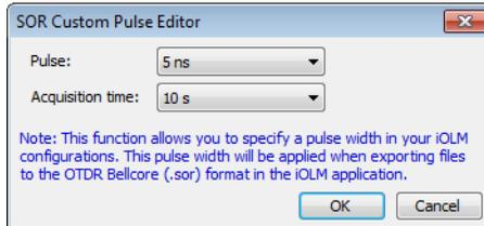
**Note:** If no pulse value is available, the pulse and acquisition time are set to “none”.
