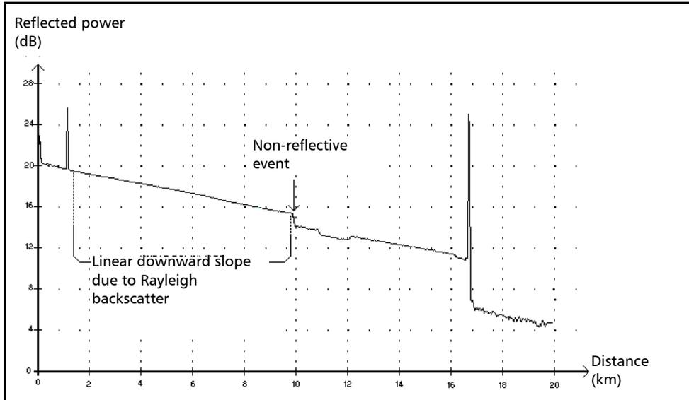
This event is characterized by a sudden decrease in the Rayleigh backscatter signal level. It appears as a discontinuity in the downward slope of the trace signal.
