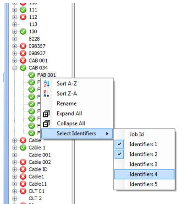
3. Select the item you wish to view in the tree. All measurements on this node, as well as those in the children nodes are displayed in the table on the right. The identifiers used in the tree view are shown in a column, you can therefore sort the results using this criterion.
