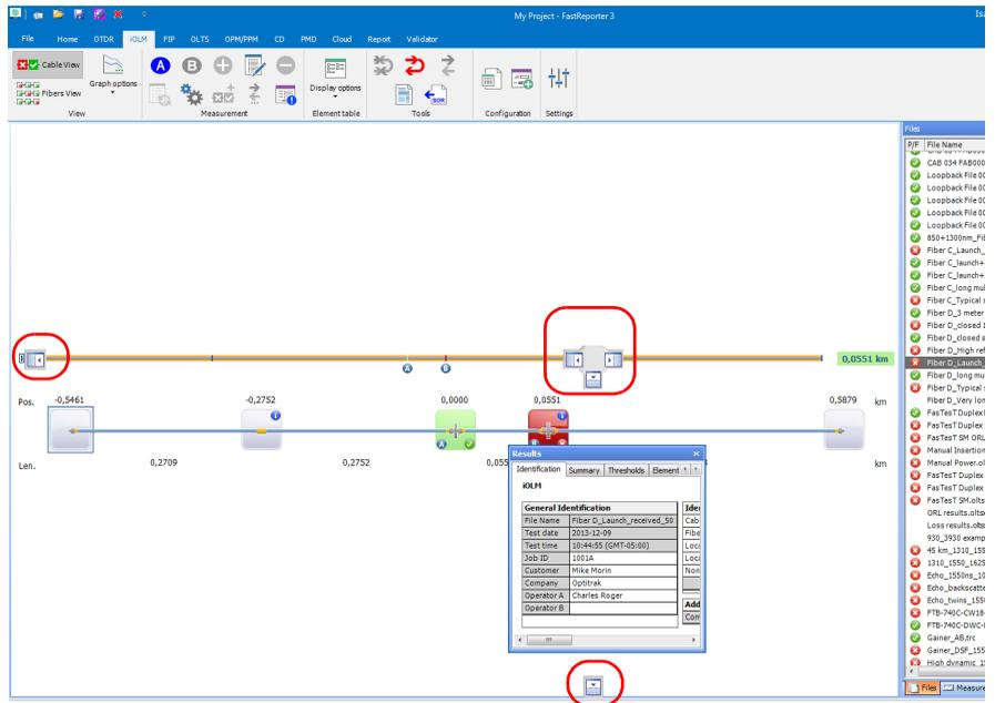
2. Drag the item from its current location to the desired anchor point, then release the mouse button.
