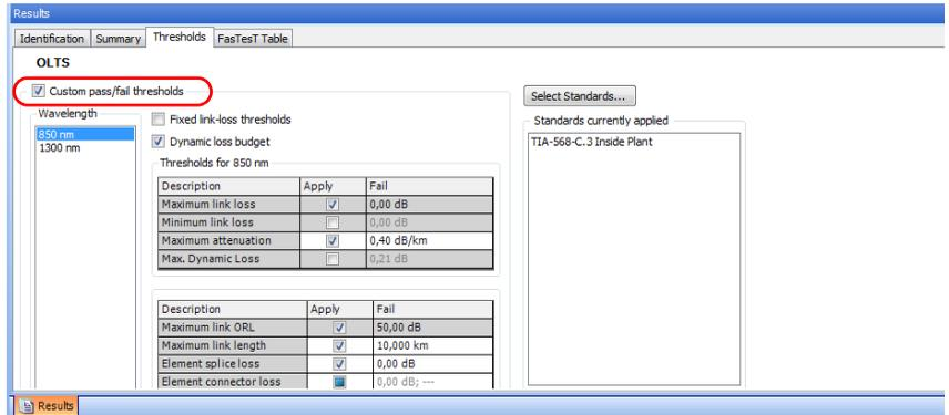
3. Select whether you want to set fixed link loss thresholds, or a dynamic loss budget, then modify the values as needed.
