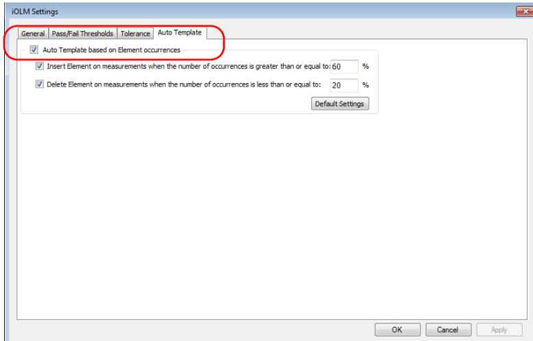
4. If you want to add elements, select the corresponding option and enter the minimum percentage value of occurrences required to add the element to the remaining links.
