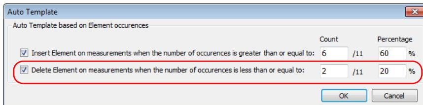
The screenshot shows the 'Auto Template' dialog box with the title 'Auto Template based on Element occurrences'. It contains two rows of options, each with a checked checkbox, a text description, and two columns for 'Count' and 'Percentage'. The second row is circled in red. The 'Count' column shows '2' and '/11', and the 'Percentage' column shows '20 %'. The first row shows '6' and '/11' for 'Count' and '60 %' for 'Percentage'. At the bottom right are 'OK' and 'Cancel' buttons.
