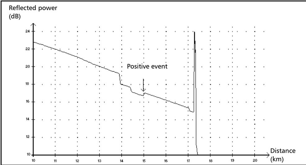
This event indicates a splice with an apparent gain, due to the junction of two fiber sections having different fiber backscatter characteristics (backscatter and backscatter capture coefficients).
