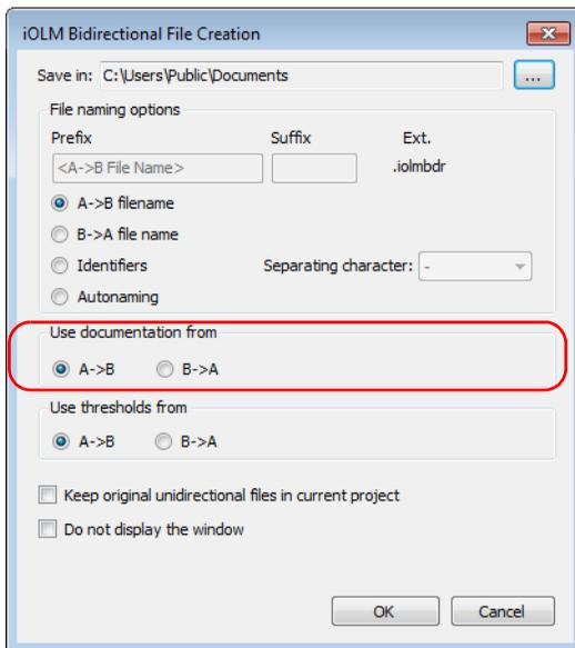
8. Select which thresholds you will use in the bidirectional measurement.
