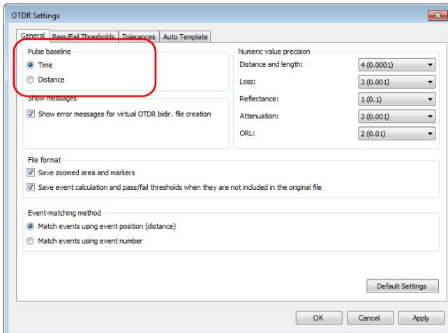
5. Change the numeric value precision settings for distance and length, loss, reflectance, attenuation, or ORL, if desired.
