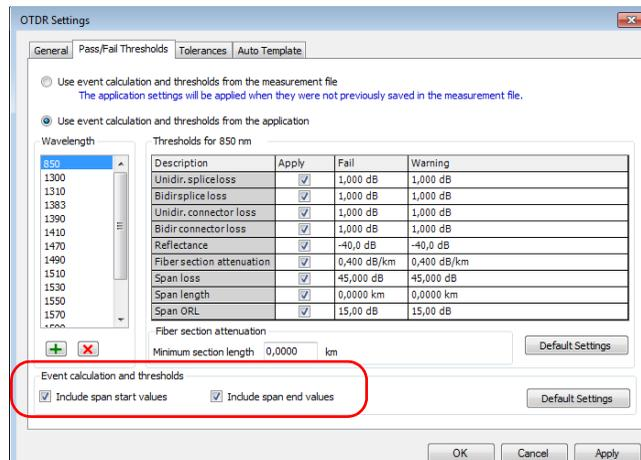
**Note:** When the span start and span end values are included, the corresponding events are included in the ORL calculation. The span start and end loss values, and the span ORL values are updated when the span start and span end inclusion settings are modified. The maximum splice loss is also impacted by the fact that the span start and end values are included or not.
