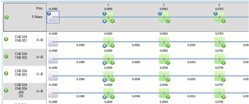
**Note:** When viewing grouped fibers, the End of fiber element (B) is set according to the reference measurement if there is one; if there is no reference measurement it is set according to the shortest fiber. The elements located between the grouped A and B positions (including both A and B) are numbered.
