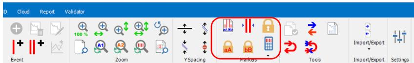
**Note:** When none of the markers are in a locked mode, you can temporarily lock the distance between all markers and move them as a block by pressing the Shift key on the keyboard and dragging them around with your mouse.
