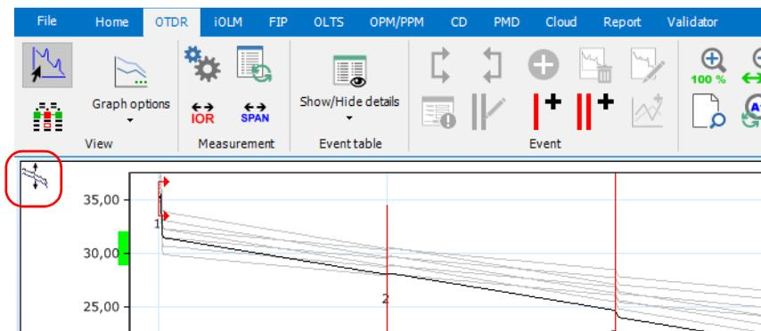
If you are using a keyboard and mouse, you can press and hold the Shift key to select the trace, then use the arrow buttons, or the mouse to drag it to the desired location.
