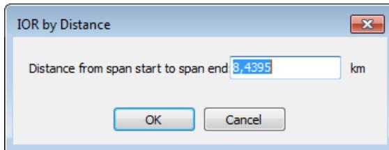
**Note:** When the distance values from the selected measurements are not the same, the values are displayed with a semicolon. Once the new IOR values are calculated, the values related to the position and distance and the OTDR graph are updated.
