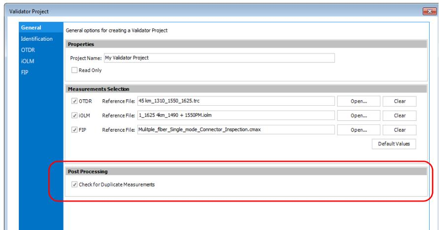
The screenshot shows the 'Validator Project' configuration window. The left sidebar has tabs for 'General', 'Identification', 'OTDR', 'IOLM', and 'FIP'. The main area is titled 'General options for creating a Validator Project'. It contains three sections: 'Properties', 'Measurements Selection', and 'Post Processing'. The 'Post Processing' section is highlighted with a red box and contains a checked checkbox for 'Check for Duplicate Measurements'.
