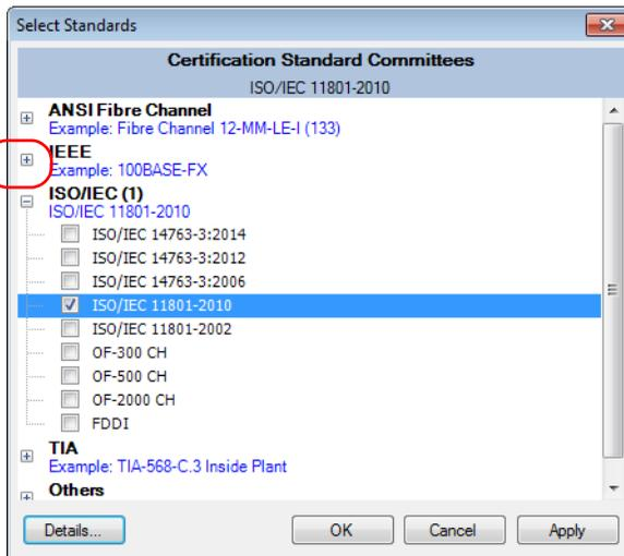
4. If you want to see the threshold details for a specific standard, select it, then click **View Threshold Details** at the bottom of the window.
