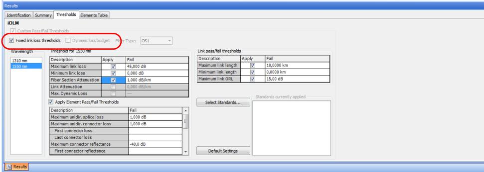
5. Select the wavelengths for which you want to view or modify the maximum and minimum loss, and maximum attenuation loss values, then change the values as needed.
