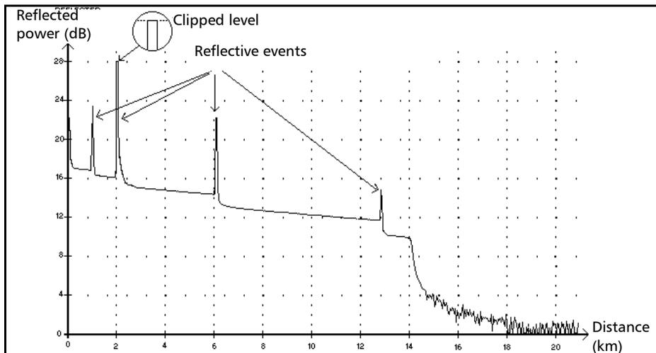
Reflective events appear as spikes in the fiber trace. They are caused by an abrupt discontinuity in the index of refraction.
