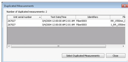
5. By clicking **Select Duplicate Measurements**, you will automatically pick the detected files in the **Measurements** tab.
