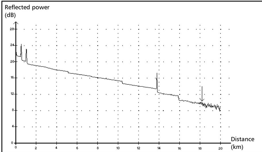
This event indicates that the pulse width used did not provide enough dynamic range to get to the end of the fiber.
