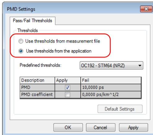
4. Modify the displayed values as needed if you selected to use a threshold from the application. The **Apply** option must be enabled for the values to be active and modifiable.
