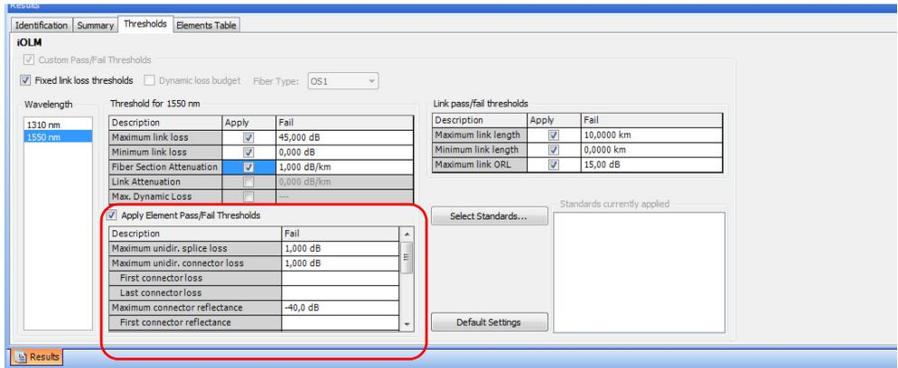
7. If the files are iCERT, you can select one or more certifications, as explained in the procedures following this one. This will display the threshold values associated with this particular type of certification. You cannot modify the thresholds displayed for them.
