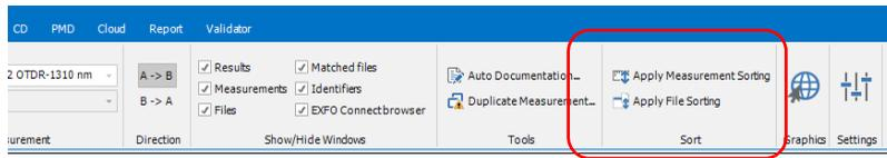
**Note:** When files in the **Matched Files** tab are not of the same type and the sorting is based on the **Files** or **Measurements** tabs, it may be possible that the sorting is not exactly the same, as priority is granted to file type and priority.
