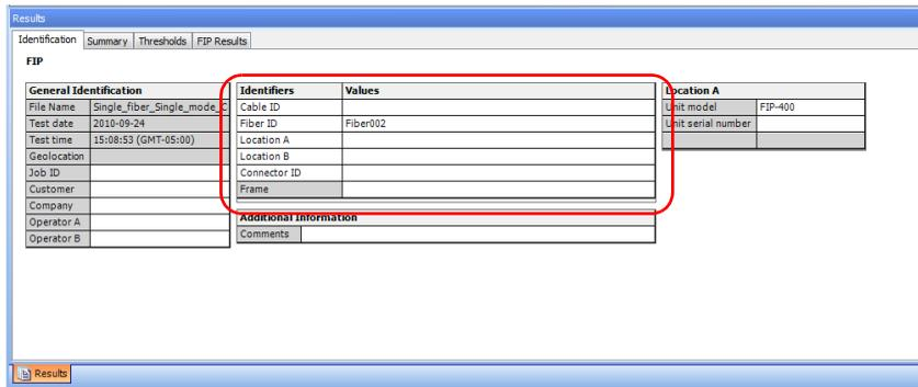
The Frame identifier type cannot be modified. Enter the information that describes the groups of connectors included in the frames, as needed.
