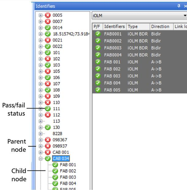
The identifier information used to sort the measurements are found under their respective **Identification** tabs. Each identifier down the list in the table creates a node in the tree. The identifiers used for matching the files are those you have selected as active in your project settings. See *Matching Files* on page 49 for more information.
