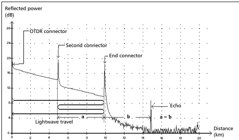
This symbol indicates that a reflective event has been detected after the end of the fiber.
