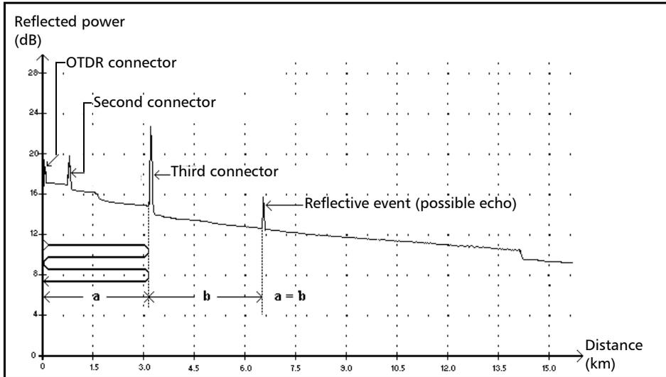
This symbol indicates a reflective event that can be a real reflection or an echo produced by another stronger reflection located closer to the source.
