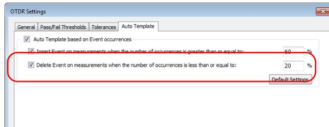
6. To apply the changes without closing the dialog box, click **Apply**. To apply the changes and close the window, click **OK**.
