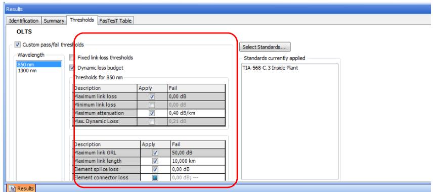
**Note:** If the unit used to take the measurements was not a Fiber Certifier (iCERT model), you cannot select the dynamic loss budget option or any of the certification standards and the maximum dynamic loss value is not displayed in the tab.
