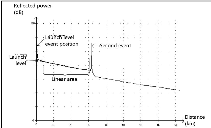
This event indicates the level of the signal launched into the fiber.
