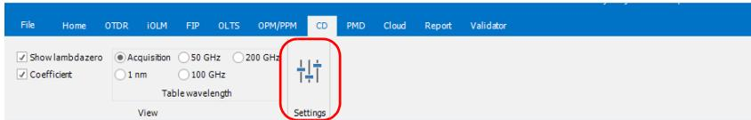
5. Select the type of threshold to use for your analysis, either from the measurement file itself or from a list of predetermined thresholds.
