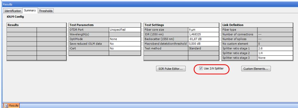
The screenshot shows the 'Results' window with the 'Summary' tab selected. The 'IOLM Config' section contains four tables: 'Results', 'Test Parameters', 'Test Settings', and 'Link Definition'. Below the tables are three buttons: 'SOR Pulse Editor...', 'Use 2:N Splitter' (which is checked and circled in red), and 'Custom Elements...'. The 'Link Definition' table shows 'Splitter ratio stage 1' set to '2:8', 'Splitter ratio stage 2' set to '1:4', and 'Splitter ratio stage 3' set to 'None'.
