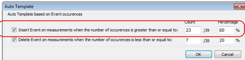
4. If you want to remove events, select the corresponding option and enter the value of occurrences under which the event must fall to be remove it from the measurement.
