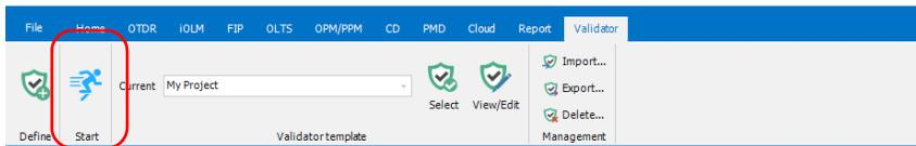
**Note:** The button is available if a template is selected and if at least one valid measurement is selected in the **Files** tab.
