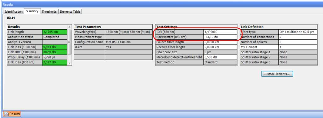
The screenshot shows the iOLM software interface with the 'Test Settings' table highlighted. The 'IOR (850 nm)' and 'Backscatter (850 nm)' values are circled in red. The 'Test Parameters' table shows 'Wavelength(s)' as '1300 nm (9 μm); 850 nm (9 μm)' and 'Configuration name' as 'MM-850+1300nm'. The 'Link Definition' table shows 'Fiber type' as 'OM1 multimode 62.5 μm' and 'Number of connections' as '2'.
