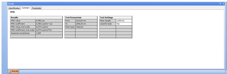
4. Locate the fiber length value under **Test Settings** and modify it as needed.
