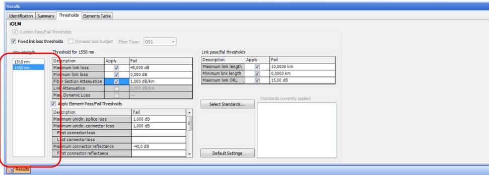
6. Enable the element pass/fail thresholds option to be able to modify them and apply them, then change the values as needed.
