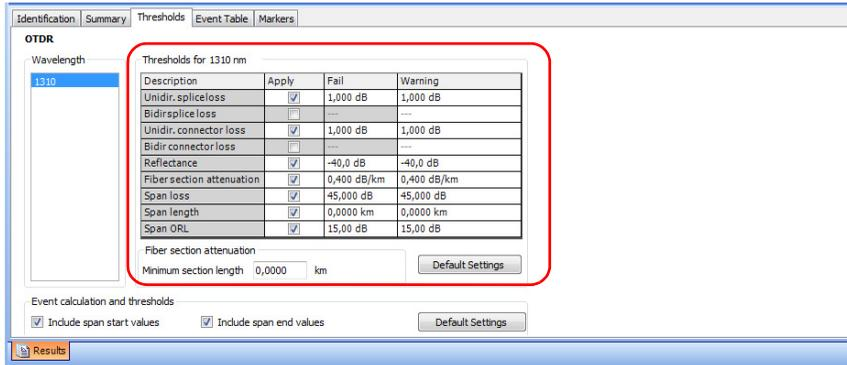
**Note:** If you are using the fiber attenuation section threshold, you can specify the minimum section length at the bottom of the table. This can be useful when testing short links, as attenuation measurements on them can be unreliable. The fiber section threshold will not be applied to fiber sections shorter than the length you have set as a minimum value.
