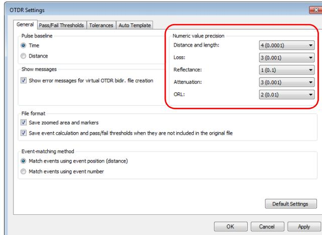
**Note:** *The numeric precision in the linear view does not apply if the selected units are meters or feet.*
