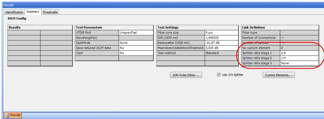
In the iOLM file, you can view the 2:N splitter value in the Link composition, and select the element type as 2:N splitter if the selected measurement supports the 2:N splitter values.
