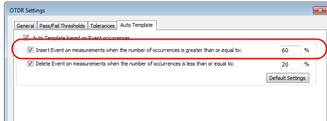
5. If you want to remove events, select the corresponding option and enter the percentage value of occurrences under which the event must fall to be remove it from the measurement.
