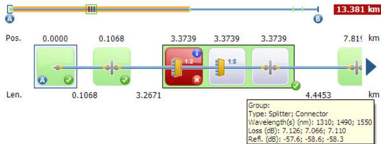
When you hover the mouse over any element with a diagnostic label, the application displays the description.
