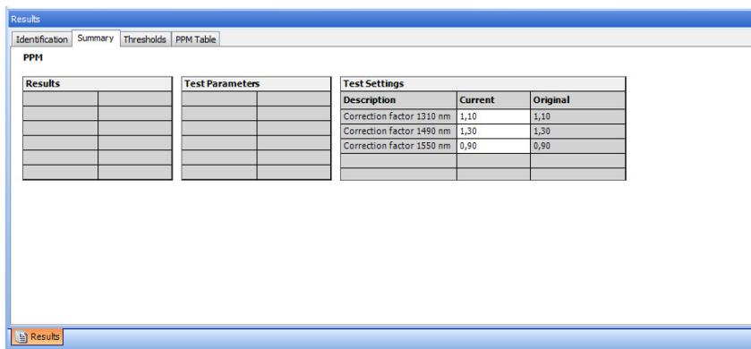
4. Modify the correction factors associated with the wavelengths as needed. Click the desired correction factor value under **Test Settings** column and modify it.
