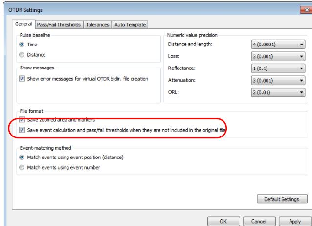
9. Select how the events will be matched, either using the position (the distance on the fiber), or the event number. The span start is considered as event number 1, or the start position.
