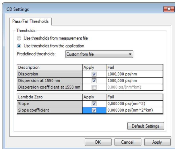
6. Modify the displayed values as needed. The **Apply** option must be enabled for the values to be active and modifiable.
