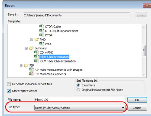
**Note:** By default, the file type is selected as Excel (\*.xls) when you run the application for the first time. The templates displayed on-screen depend on the file type you have selected.
