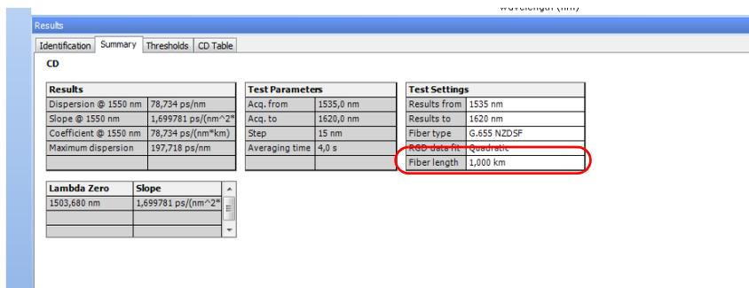
**Note:** If your file is in .cdpmd format, the fiber length was measured automatically during the measurement and cannot be edited.
