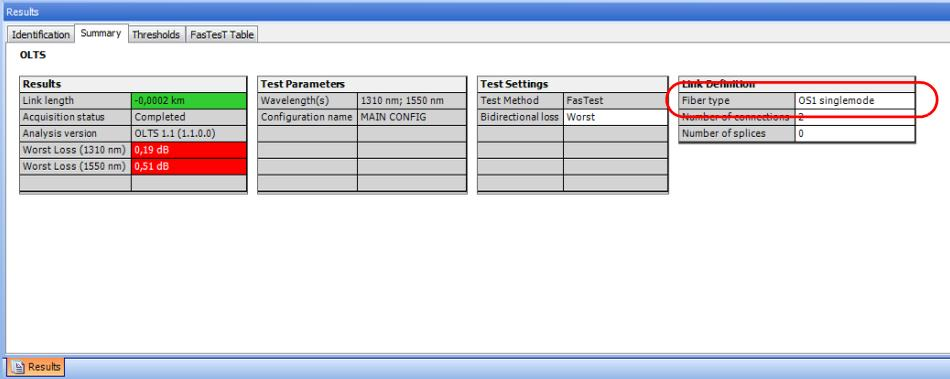
The screenshot shows the Results software interface with the Summary tab selected. The OLTS section contains four tables: Results, Test Parameters, Test Settings, and Link Definition. The Link Definition table is circled in red, showing the Fiber type set to OS1 singlemode.
