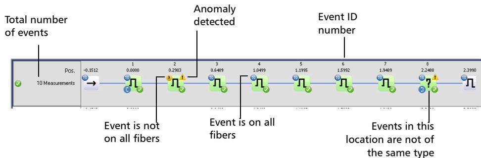
**Note:** When viewing grouped fibers, the Span End event (B) is set according to the reference measurement if there is one; if there is no reference measurement, it is set according to the shortest fiber. The events located between the Span Start and Span End events (including both A and B) are numbered.
