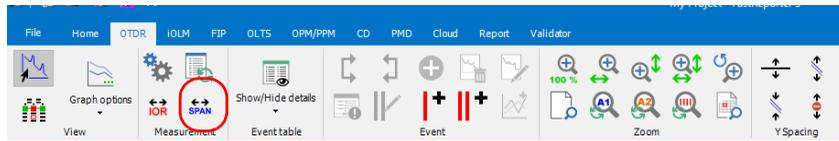
4. Set the launch fiber length as required. Once you set the launch fiber length, the application updates the span start position and span length value based on the new position of the span start. If no event is present at the new position of the span start, it automatically creates a new event.
