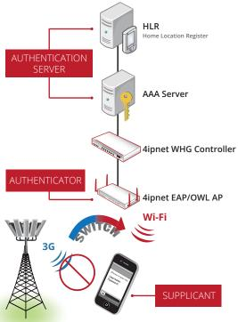
explosion of mobile device traffic in recent years, carriers are increasingly using EAP methods such as EAP-SIM and EAP-AKA to automatically offload clients from their 3G networks to Wi-Fi.
