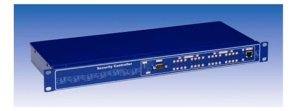
The PVMax Security Controller enables control of a variety of sensors and remote-controlled devices from the PV4E Management Station. Sensors such as temperature, humidity, floods etc., and remote devices such as rack indicators, door locks, door switches, fans, can be physically connected to the PatchView system using the PVMax Security Controller. The PVMax system also uses secure communication in order to avoid unauthorized access.
